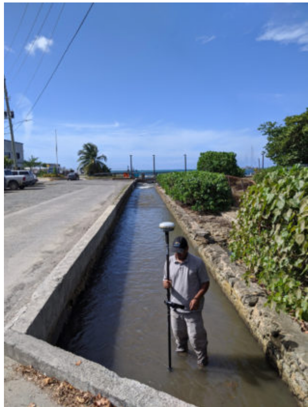
Greg Guannel, director of UVI's Caribbean Green Technology Center, measures sediment depth in the gut that empties near the seaplane terminal in Christiansted. (Photo submitted by Hilary Lohmann, DPNR)
